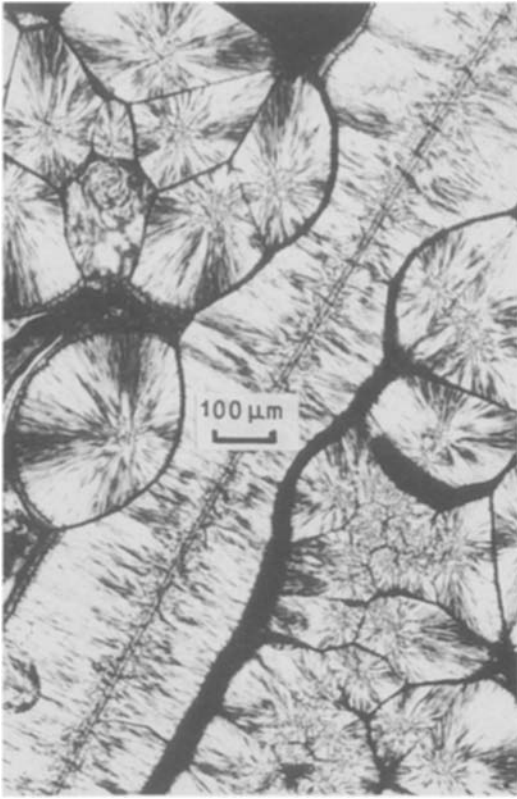
Figure 10 Twaron/PP pulled 1 \text{ mm min}^{-1} , T_c = 140 \text{ }^\circ\text{C} .
