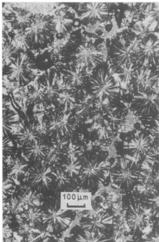
Figure 14 Twaron/PP cooled at 1 °C min -1 .
